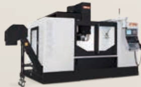
HMC series Horizontal Machining Center (with pallet change system)
